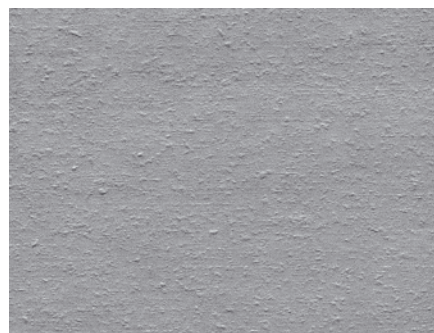
FIGURE 7: Intensity-encoded slope of a flake board. The small dents are about 3 microns high.
